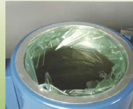
LSJRE boiling chamber filled with solvent.
