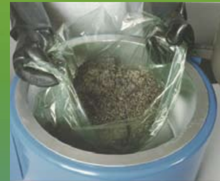
Residue is removed from the boiling chamber at process completion and disposed of according to local regulations.
